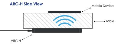
The ARC logo & magnet on the underside of the ARC-H indicates the centre of the charging coil. Ensure the unit is mounted aligning the desktop decal with the arc logo.
